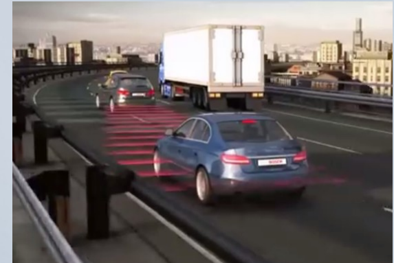
Fahrerassistenz-System Adaptive Cruise Control (ACC). Bild: Bosch – [on-line]: https://www.youtube.com/watch?v=own_VaRZ9M8
